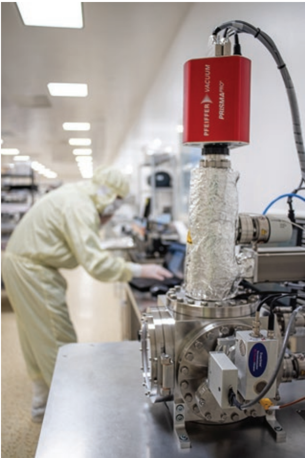
Plasma cleaning device with RGA Analysis
