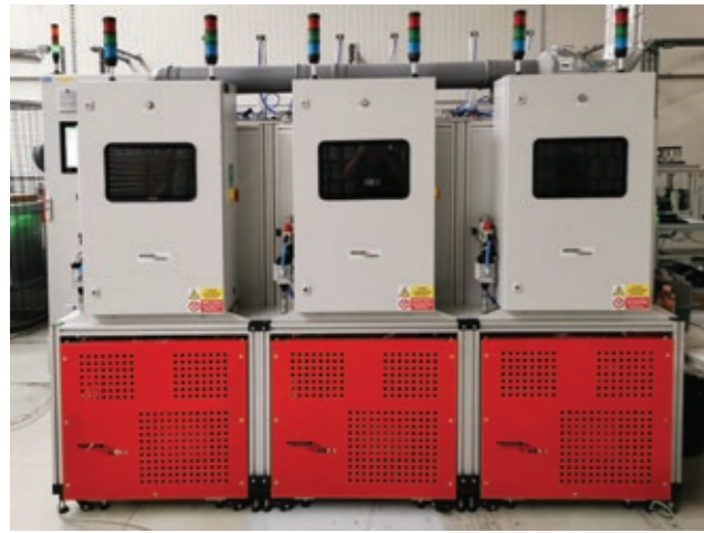
Parallel HLDS configuration for Valve leak testing
