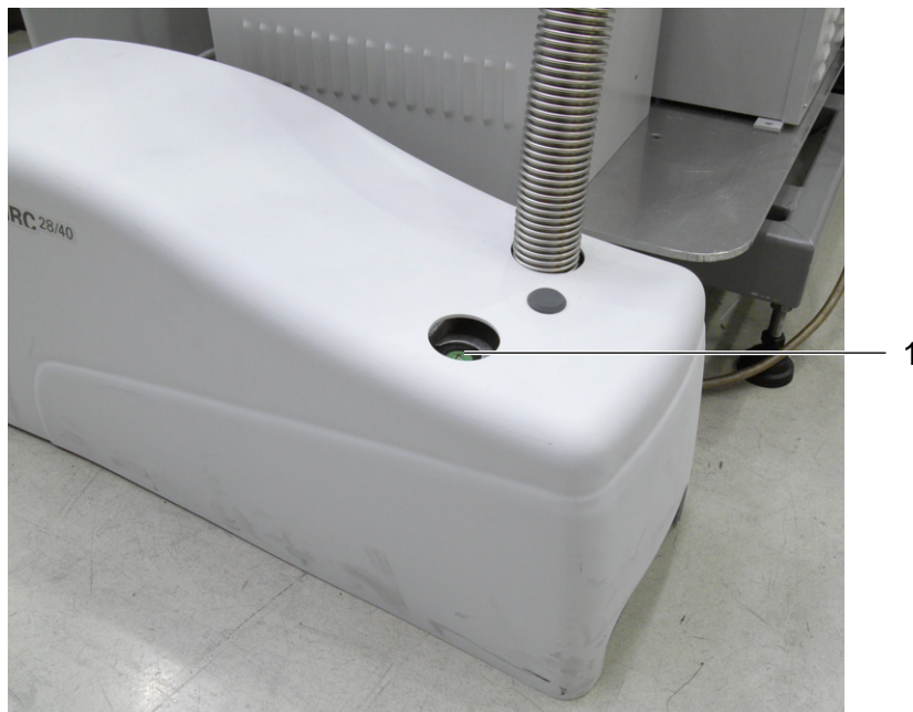
Fig. 9: Exhaust connection at the backing pump
