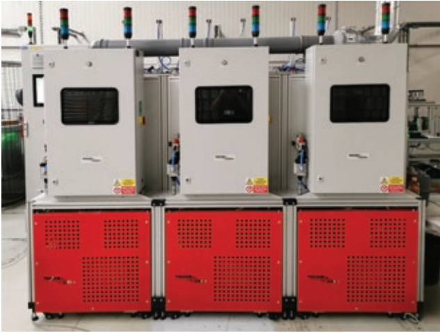
Parallel HLDS configuration for Valve leak testing
