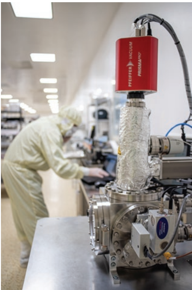
Plasma cleaning device with RGA Analysis
