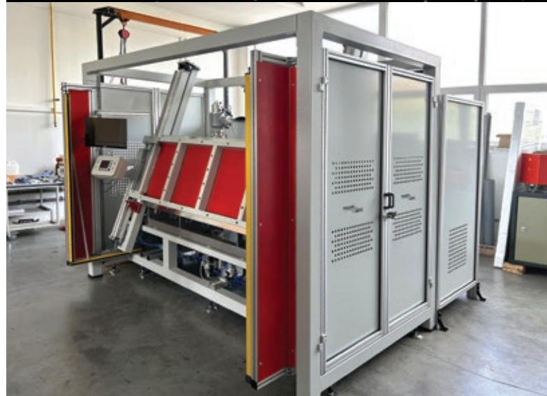
HLDS for high pressure AC components
